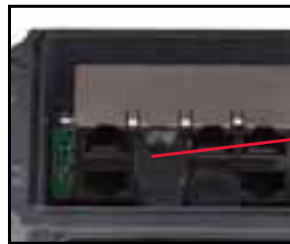
8-Way Connector Bank for SCI Cable Assembly to Switches
